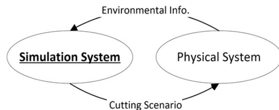
Fig. 1. Concept of the dismantling control system.
